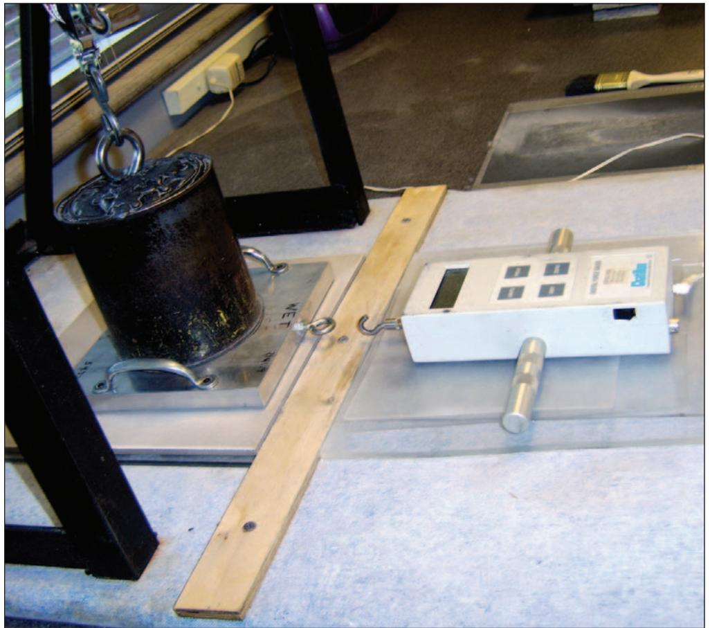
*This is a horizontal dynamometer pull-meter testing assembly and weight, sitting atop a tile being tested at the TCNA laboratory.*
