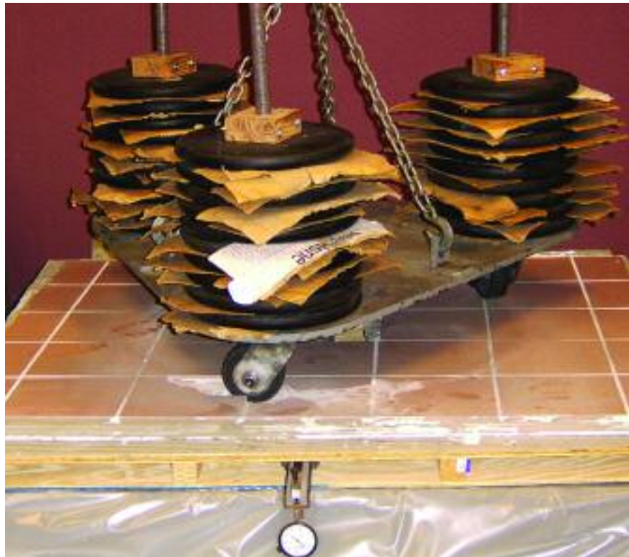
Right: The Robinson-type floor test provides data that determines a floor's rating. Photo courtesy of TCNA Lab.
