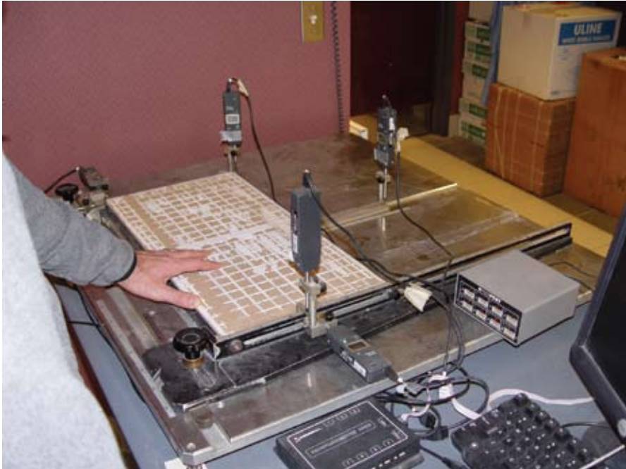
Potential ANSI A137.1 revisions to evaluate tiles based on individual measurements of edge warpage could further improve the way rectangular tiles are measured and reported.
