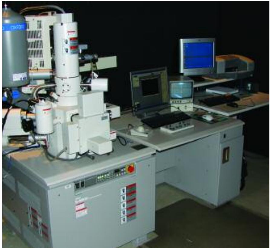
A scanning electron microscope gives three-dimensional images over a wide range of magnification, allowing examination and measurement of surface features such as cracks, pits, and inclusions. Photo courtesy of Clemson University.
