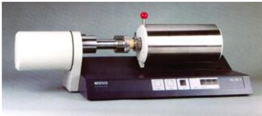
The dilatometer measures size changes (expansion and/or contraction) with changes in temperature. This is especially important to determine if tile bodies and the glazes applied to them "fit" each other and to determine if internal stresses could be created by the firing and cooling process. (Image courtesy of the NBRC)
